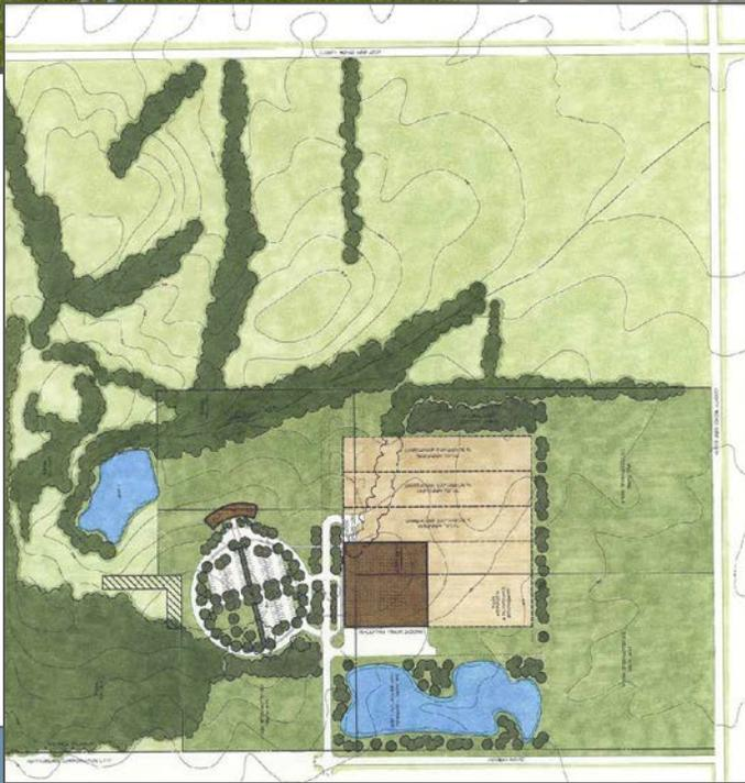
Architecture Plus developed a master plan for a 50-acre site in Huntingburg, Indiana, on which a new 600,000 square foot warehouse -office facility was developed. The master plan included phases I, II, III and IV for planned warehouse expansions. The first construction phase is shown. The facility utilized tilt-up concrete wall construction.
